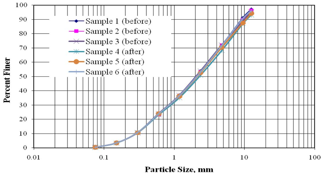
**Figure 2. Gradation Curves of the Aggregates Extracted by the Ignition Method Before and After Compaction**
